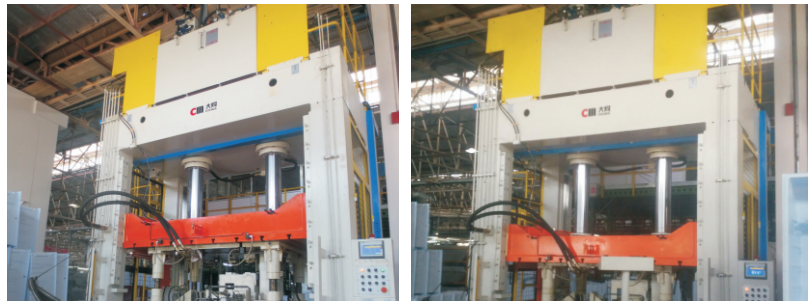
冰箱内胆专用打孔及裁边油压机 Refrigerator liner trimming and punching hydraulic press
