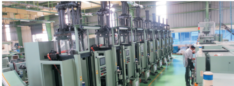
管材冷挤压成型伺服油压机生产线 Servo driven hydraulic press production line for cold extrusion tube forming
